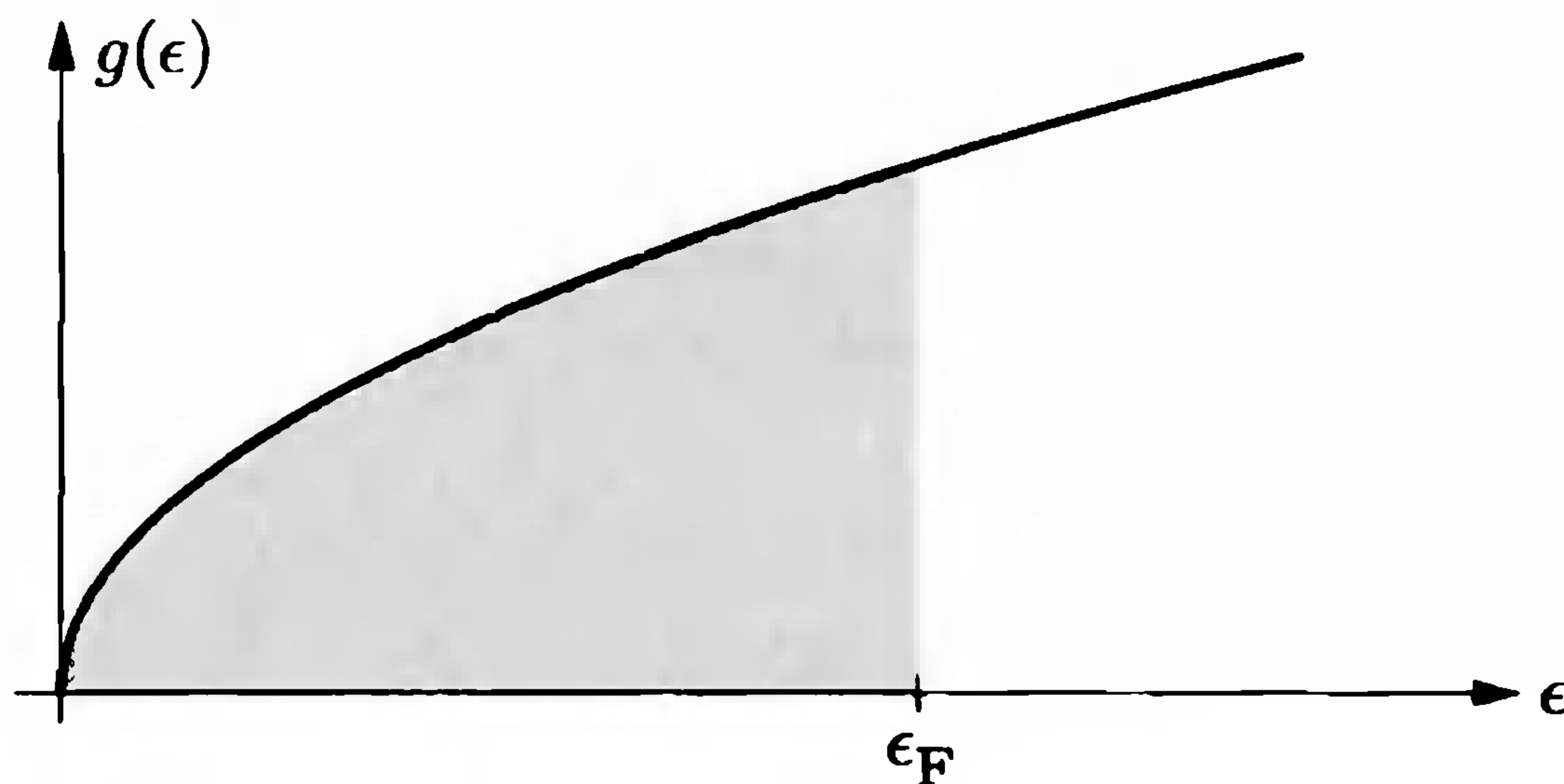
Figure 7.13. Density of states for a system of noninteracting, nonrelativistic particles in a three-dimensional box. The number of states within any energy interval is the area under the graph. For a Fermi gas at T = 0 , all states with \epsilon < \epsilon_F are occupied while all states with \epsilon > \epsilon_F are unoccupied.
